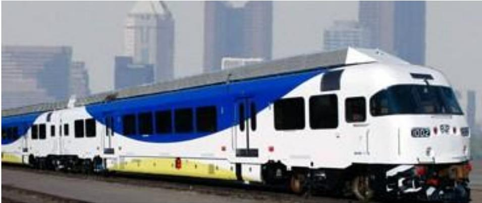
Figure 2. **Single-level Diesel Multiple Unit (DMU) to be manufactured by US Railcar in Ohio.**
